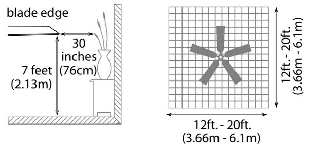
This fan can be mounted with a **downrod** on a regular (no-slope) or vaulted ceiling. The hanging length can be extended by purchasing a longer downrod (0.5in./1.27cm diameter). *After installing hanging bracket, continue to Section 5 on page 4 for those instructions.* This fan can also be mounted as a **flushmount** on a regular (no-slope) ceiling. *After installing hanging bracket, continue to Section 6 on page 5 for those instructions.*
