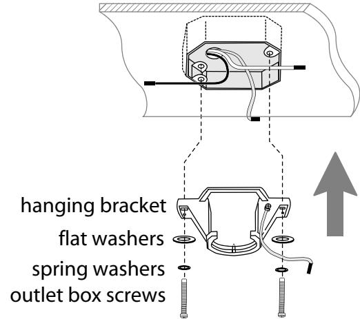
**\*Note:** It is very important that you use the proper hardware when installing the hanging bracket as this will support the fan.
